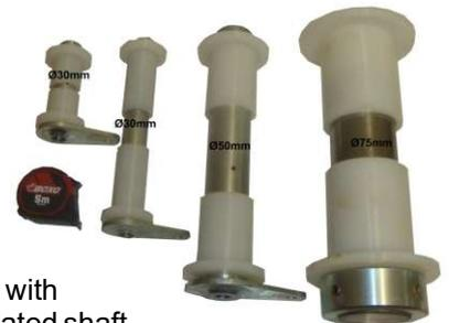
Caster wheel and bogie rocker pivots are Ø75mm shaft.
