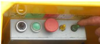
CAGE is enclosed on three sides, safely protecting the operator from branches. Also sited in the cage is (L-R) electric throttle, E-Stop, Start, Bin Forks, Electric Hydraulic Three Speed, Horn & E-Decent. All switches are rated IP67 and sealed in an aluminium box.
