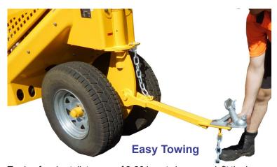
Towing for short distances of 2-20 km at slow speed: fit the heavy duty draw-bar; push the free-wheel pin in the planetary hub in, then rotate 90°. Page 4 of 9
