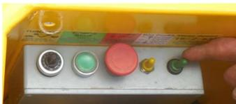
CAGE is enclosed on three sides, safely protecting the operator from branches. Also sited in the cage is (L-R) Electric Throttle, E-Stop, Start, Electric Hydraulic Three Speed, Horn and E-Decent . All switches are rated IP67 and sealed in a box.
