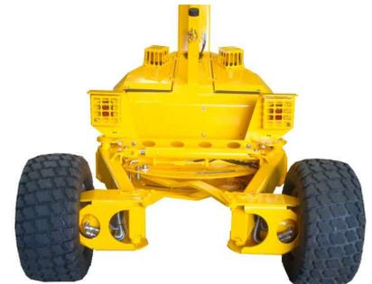
**Hydraulic Swing out drive wheels width 1.75m - 3m**
