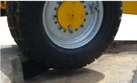
The larger wider wheels make driving over street kerbs large branches and soft ground a lot easier and smoother, enabling the operator to continue driving and pruning efficiently. On the right side of each picture is what most other makes of EWP's use.
