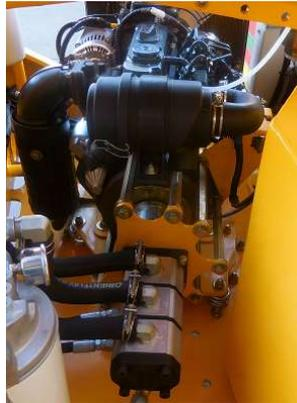
**Kubota diesel engine 23hp 3 cyl water cooled**
