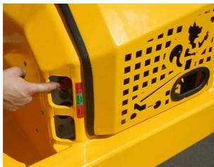
E - Stop and Start & E-descent switch, are accessible without lifting the bonnet.
