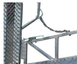
2 gas struts, heavy duty latch and check chain lock rear ramp up.
