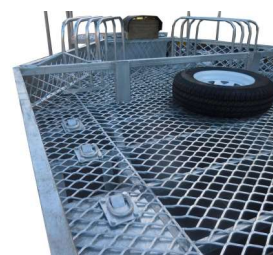
14 tie down lugs on tray and rear slope, for tying down any machinery
