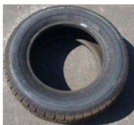
Heavy rated tyre, 225/75R15 x 10 ply load rated 117/112, for 2021 & 2023 trailers TRT225/75R15-10 $130.02 + GST
