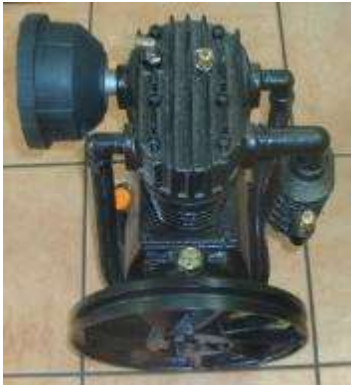
Compressor 6cfm heavy duty, 2 cyl two stage, 175 psi, head unloader, Cast iron Flywheel 10½" A section – CCFH20T
