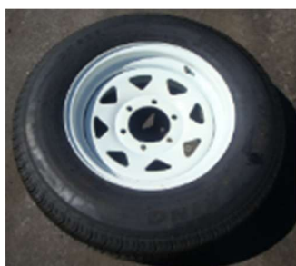
Wheel, 195R15C tyre in 15" rim, Land Cruiser 6 x at 139.6 PCD Tyre 8ply tyre: for 2021 & 2023 trailers TRW195R15C+15 $251.87 + GST
