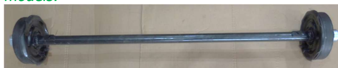
HD Trailer axil Ø65mm, solid ends for 0.4m hollow in centre for 1.8m, Brake hub drum 12" x 2.5", 6 x Ø1/2UNF at 139.6 PCD (Land Cruiser) with bearings. Wheel nuts, dust caps, rated at 4.5ton for double axil trailer usage, for 2021 & 2023 trailers; AHASWHDB12X2.5 $939.23 + GST
