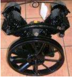
Compressor 22.4cfm 2 cyl single stage head unloader ZL2080H (picture right) – CCZL2080H
