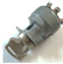
D902 Engine key assembly (after market); 1E013-63593AM $57.60 + GST
