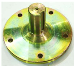
Kubota engine drive shaft Ø35mm, 10mm keyway for all Kubota engine, (from 7-2024)- EKD902SS35
