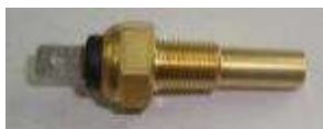
Kubota D902 Engine Water temperature sender switches light on when water is too hot, we connect to stop engine so that it is failsafe overheat engine stop (genuine) D722 – D902 16222-83041
