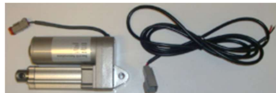
Linear actuator heavy duty 700N; 40mm stroke; 12V black lead with deutsch plug x 2.5m, IP66 (Electric throttle from mid-2021) – LA100IP66-LAJ $111.82 + GST (This is what we are using now)
