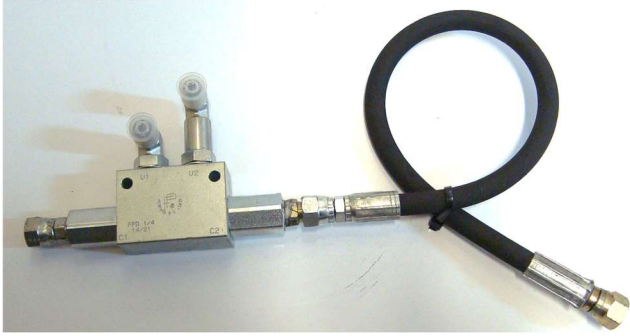
Double pilot check valve ¼" kit and hose for side swing of bin forks ram, 9/16 JIC, stops ram creeping – RDPCV14KAH*
