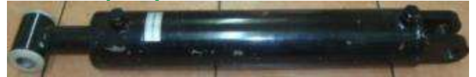
Ram 406mm travel, 90mm piston, 50mm pushrod, bottom 30mm pin, top boss 78mm long with 38.15mm hole, no HDPE bushes fitted (355 & 505 from 2016) – RCHM406x90x50 $809.00 + GST
