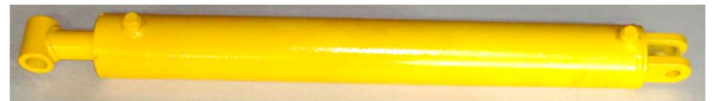
Ram 762mm travel, 90mm piston, 50mm pushrod, 1" bottom pin, top boss 95mm long with 38.15mm hole, no HDPE bushes fitted (pre-2016, 655 & 805) – RCH30X3.5X2
