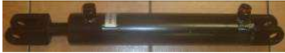
Ram 205mm travel, 65mm piston, 32mm push rod, 1" pins (3.8m SS) – RCH205X65X32
