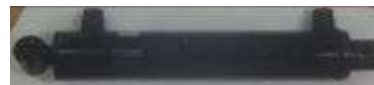
Ram 254mm travel, 50mm piston, 25mm push rod, 40mm, boss both ends with 20.5mm hole (Side Swing Ram up to mid-2014 & all Bin Forks ram) - RCHM10x50x25 $354.00 + GST
