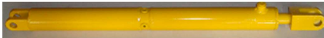
Ram 975mm closed – 1280 open, 305 travel, 63 piston, 36 push rod, 1" pins painted with 4 x 3/4" UNO ports (for 655 & 805 drive wheel retraction) – XHWR* $576.00 + GST
