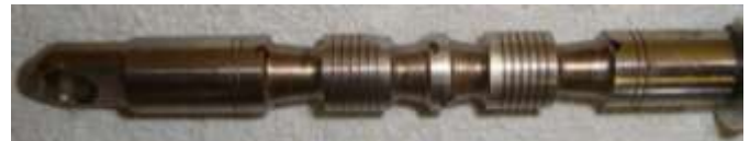
Lift valve Spool, (double acting cylinder ground down for lift ram); Galteck Q45) – XSLRG*
