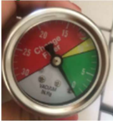
Suction Filter stainless steel glycerine filled vacuum gauge Ø40mm 1/8" BSPT – FHSFVGSSG
