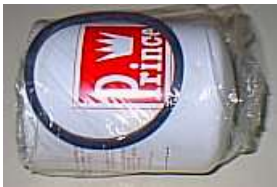
Filter hyd Element only, 10-micron, PRINCE FB10, 1 1/2-16 UN-2A internal thread, 125mm diameter 170mm long – upgraded to 140mm diameter 190mm long FHFB10 $64.80 + GST
