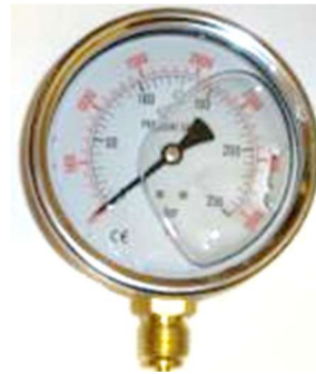
Ø100mm glycerine filled gauge 3,600 psi/250 bar, 1/2" BSPP Part number GGP100250
