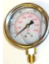
Ø63mm glycerine filled gauge 3,600 psi/250 bar, 1/4" BSPP Part number GGP3600
