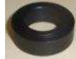
O-ring encapsulated Seal retainer 14.15x8.1mm, this seal retainer instead of the original white nylon which loses its shape when it gets hot, This black seal retainer is shorter to allow more space for wider seal, – VHCGSR1415 $9.52 + GST (Use 1 off per seals O-ring encapsulated Seal)
