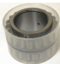
Needle roller assembly for planetary gear cog RSL185006 29.5 id x 35.3 wide reference #29 - IF20-NRAFPGC
