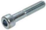
Danfoss Socket head cap screw 6 x 30 to hold bearing cap plate in hub, 10 required to replace set, These can be stretched when hub is pressurised, – BSHCM06X30
