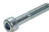
Danfoss Socket head cap screw 6 x 30 to hold bearing cap plate in hub, 10 required to replace set, Theas can be stretched when hub is pressurised, – BSHCM06X30
