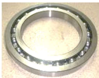
Renold main bearing 2 required 160 od x 105 id x 18 wide – B16021
