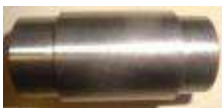
Planter cog-centre shaft V565 #24, 8:1 reduction CM#7 hub, Ø21.2, ends Ø19 x 45 total length (after 11-2015) - AHPWD565SGCCS24
