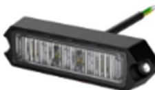
Amber LED flashing strip 10-30V, IP67, 36w, 47mm 132 long x wide x 18mm height LH212– EGSLLEDA $37.68 + GST
