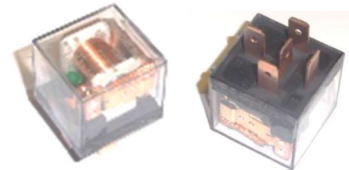
Relay 5 pin. double reversing contact 12V 40A, very HD, clear body, LED light when operating (from 5-2025) - ESRR12V100A $4.26 + GST
