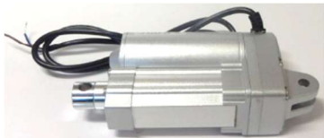
Linear actuator heavy duty 700N; 40mm stroke; 12V black lead 1m, IP66, has slot in foot mount (Electric throttle from mid-2026) – LA100IP66SYAO4B $..... + GST
