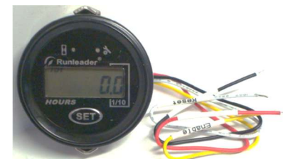
Hour meter LCD, maintenance minder, programable can pre load hours on it, can see number when engine is off, 20year life, IP67, Ø51 hole 5/36V, DC (new from early-2025) - HMIP67RL069A $67.52 + GST (This is what we are using in-2025)
