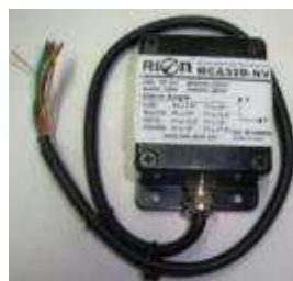
Tilt switch 2 axis, 4 fixed alarm 7.5° & 10°, 12.5° & 10°, 12.5° & 15°, 15° & 17.5°, 2 sec delay 0° set (0.6m lead), 3 amp - EMSMCA32D-NV (up to 2-2025)
