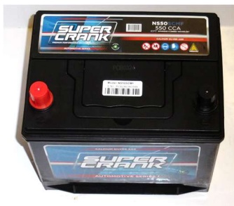
Battery 550 CCA, big terminals, 170mm deep x 230mm wide x 210mm high (for diesel 008 models)- BASC550 $148.88 + GST
