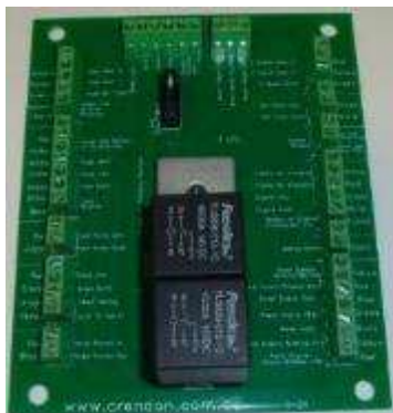
PCBA wiring board – 008 series; Squirrel 3 Speed: height cut-in for slope sensor, height cut-out on 3 speed, starter solenoid, 2 x live circuits, plug in diode, bridge rectifier. (from 2021) - PCBA-SQ21
