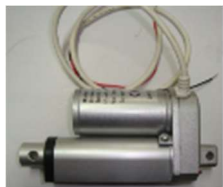
Linear actuator light duty 200N; 40mm stroke; 2.5m lead, IP65 (Electric throttle before 2019) – LA40N40S12V $54.91 + GST
