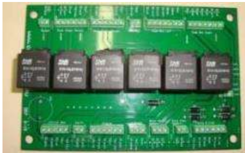
PCBA wiring board - 007 series; Squirrel 3 Speed: drive wheels position, height cut-in for slope sensor, height setting for slope sensor settings, oil pressure buzzer, height cut-out on 3 speed, starter solenoid, bin forks, crab steer, boom sequence, (from late 2015) - PCBA-SQ007
