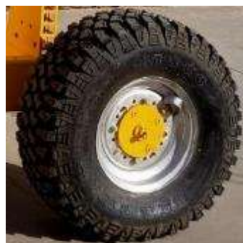
Wheel complete: 33" x 12.5" – 15" x 6 ply 4x4 tread on 15" x 8.5" 10mm centre, 60mm of center, 16 x Ø16 counter sunk holes at 220 PCD, valve guard, hot-dip galvanised rim (for drive wheel 508 & 708 before 2024) - TRW33*12.5-15GC4X4T
