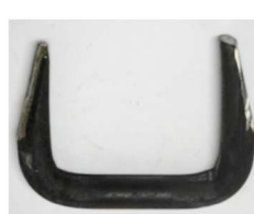
Boom cage end reinforcer Ø24mm rod, ends taper off, bent in U shape to go around top of boom opening–
