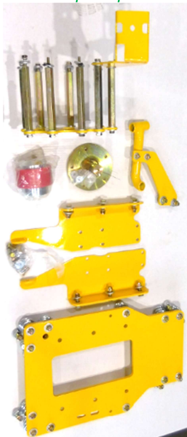
Kubota D902 Engine base kit with base plate up to and including 2015, hydraulic pump bell housing, Engine to hyd pump cupping # CSRF55-115-35R, 2 x bell housing stand of extension 20mm hex spacers 10mm FM thread one end 8mm FM thread other end for air cleaner, 7 x bell housing stand of extension 20mm hex spacers 10mm FM thread both ends, throttle mount bracket, radiator mount, engine stands, Ø35mm stub shaft with 10mm key, exhaust extension pipe, exhaust clamp, all bolts, 12 engine springs; EKD902EBK* $1,119.80+ GST
