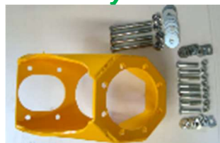
Drive hub bracket for 505 from planetary wheel hub to RHS frame all made from 10mm plate includes all HT bolts & washers – XSDHB505*
