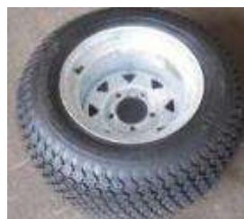
Wheel complete Tyre & Rim, 560mm Ø x 300mm wide, (for 358 Squirrel 2020 to 2025) Rim 12" x 8.5" ford PCD, 12mm offset, hot dip galvanised fitted with Tyre 22 x 12 x 12, 4 ply – TRW22X12X12X12GAL
