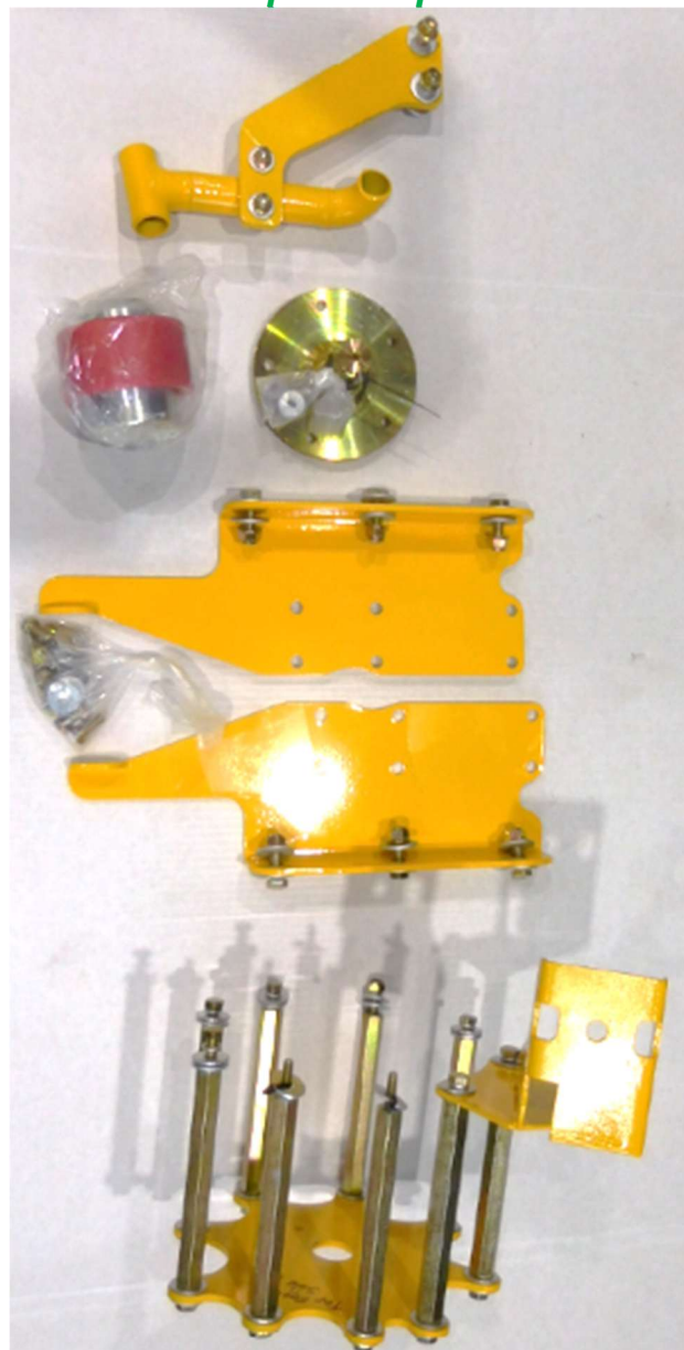
Kubota D902 Engine brackets kit without base plate, hydraulic pump bell housing, Engine to hyd pump coupling # CSRF55-115-35R, 2 x bell housing stand of extension 20mm hex spacers 10mm FM thread one end 8mm FM thread other end for air cleaner, 7 x bell housing stand of extension 20mm hex spacers 10mm FM thread both ends, throttle mount bracket, radiator mount, engine stands, Ø35mm stub shaft with 10mm key, exhaust extension pipe, exhaust clamp, all bolts, no engine springs; EKD902EK* $840.28 + GST
