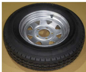
Wheel complete: 165R13 8 ply road tread on 13" x 4", 0mm of centre, 5 x Ø15 counter sunk holes at 114.3 PCD, Ford PCD, hot-dip galvanised rim, (for caster wheel 358 from 2025) – TRW165R13+RHDG $..... + GST
