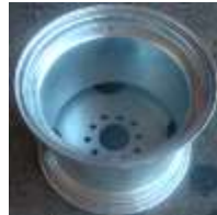
Rim 12 x 8.5 Orchard chain drive style, hot dip gal, sand blast & paint, 10mm centre, holes to suit holden HT & Ford PCD (for all chain drive)
