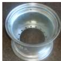
Rim Ø12"x 8.5" Renold plan hub style 16 x Ø11 holes, hot dip gal, sand blast & paint, 10mm centre, (1995 - 2004) -
