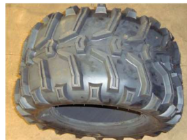
Tyre 25x12.5x12-8PR bear claw grip, t/less 8 ply - TRTBC25X12.5X12C $207.96 + GST
