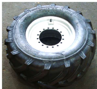
Wheel complete: 31" x 15.5" – 15" x 8 ply tractor grip tyre on 15" x 10.5" 10mm centre, 75-80mm of centre, 16 x Ø16 counter sunk holes at 220 PCD, valve guard, hot-dip galvanised rim - TRW31*15.5-15GC $535.12 + GST
