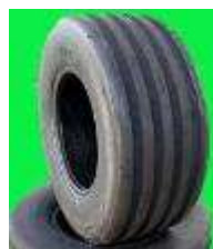
tyre 620mm Ø x 300mm wide x 12 ply, load 1200kg each, (for 558, 678, 818, 536, 656 & 806) (from mid 2018) TRT26X12X12-12P
