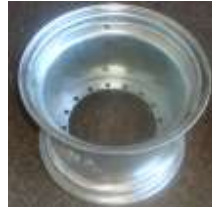
Rim Ø12"x 8.5" Renold plan hub style 16 x Ø11 holes, hot dip gall, sand blast & paint, 10mm centre, (1995 – 2004) –
