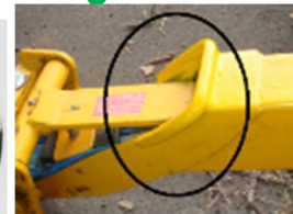
Boom cage end reinforcer Ø24mm rod, ends taper off, bent in U shape to go around top of boom opening–
