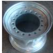
Rim Ø12" x 8.5 Crendon hub style 12 x Ø15 holes. hot dip gall, hot dip gall, sand blast & paint 10mm centre, -
