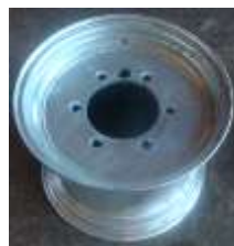
Rim Ø12" x 8.5 Danfoss hub style 6 x Ø15 holes, hot dip gal, hot dip gal, sand blast & paint 10mm centre, (2004 -
