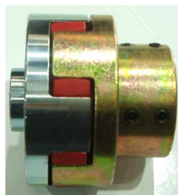
Heavy duty coupling complete, outer diameter 120mm, 1.125" with ¼" keyway and group 2 taper shaft for pump with red centre #55– CSGR551.125-120* $137.20 + GST
