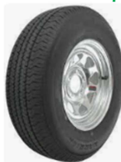
Wheel complete: 215/75R14 8 ply road tread on 14" x 5", 0mm of centre, 5 x Ø15 counter sunk holes at 114.3 PCD, Ford PCD, hot-dip galvanised rim, 1120kg load rated each (for caster wheel all 005, all 006 558, 678 & 818) - TRW215R14+RHDG $204.89 + GST
