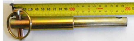
Top link pin, Ø3/4" & Ø1", with linch pin from 2017, - ZNWTLP17
