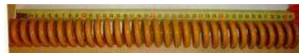
Head spring Double front mount Sadie - 1.5"ODx0.2830 wire x 400mm long - SBC1.50D0.283X4
