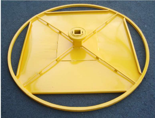
Spindle cover (1.05m) for Standard & Hi-Lift, 4mm x 300mm square reinforced center, Ø8mm rod to outside frame, center bearing held on with C-Clip – ZNWSC
