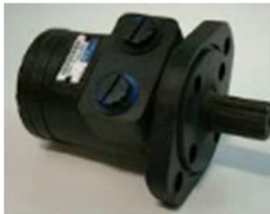
Hyd motor for worm drive gear box 80cc 2blt flange, 1" straight shaft, 1/4" keway, 7/8UNF ports, no case drain, BMPH-80-H2-K-S-B-O (from 2023) - BMPH80H2KSBO
