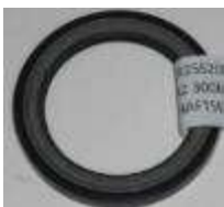
Shaft seal HP BMER-2 hydraulic motor rated to 200 bar, 35 id x 48 od x 4.72 wide – MHCBMER2SS200
