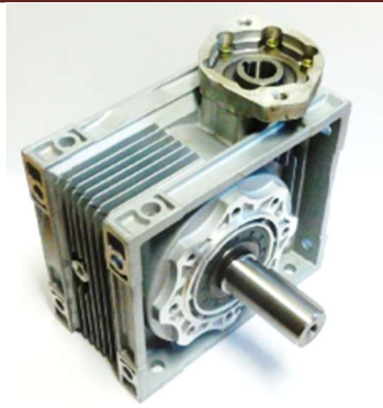
Worm drive RV90-20DZ, 20:1, input hyd motor flange, Ø35 output shaft (from 2023) – GBRV90-20DZ $713.47 + GST
