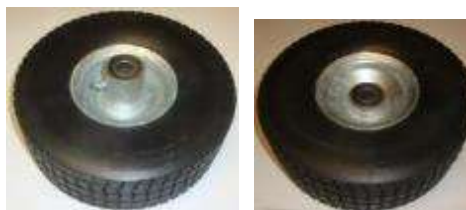
Wheel 4.10-3.50-4" air free wheel, 73mm wide tread, welded rim hot dip galvanising, with 6203-2RS bearings & spacer, no bolt axle V'yd Sadie - ZVS4WS*
