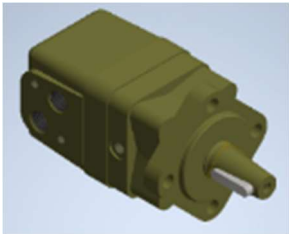
Sadie Double Sided Front Mount; Like Hyd motors BM5 100cc with tapered shaft, 4 bolt flange, 7/8UNO ports (from 2022 on) – MHCBM51004BTS
