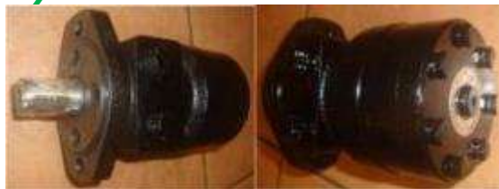
Hyd motor TPF BMRS400; 395cc, 2 bolt flange, 1" shaft with 1/4" keyway, 7/8UNF ports, low speed, high radial load, 250 bar shaft seal. (from 2000 – 2019) – MHCBMRS4002B1S $502.11 + GST
