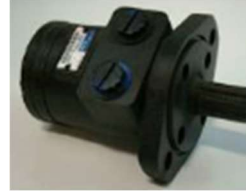
Hyd motor for worm drive gear box 80cc 2blt flange, 1" straight shaft, 1/4" keway, 7/8UNF ports, no case drain, Like BMPH-80-H2-K-S-B-O (from 2023) - BMPH80H2KSBO
