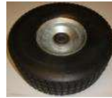
Wheel 4.10-3.50-4" air free wheel, 73mm wide tread, welded rim hot dip galvanising, with 6203-2RS bearings & spacer, no bolt axle V'yd Sadie - ZVS4WS* $..... + GST
