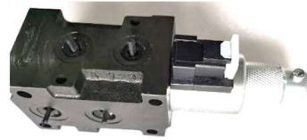
Sadie Double Sided Front Mount; Elect selector valve 6 port, 9/16 UNO ports, Deutsch solenoid IP67, manual override, (from 2019 on) – – VS6PE916DNO
