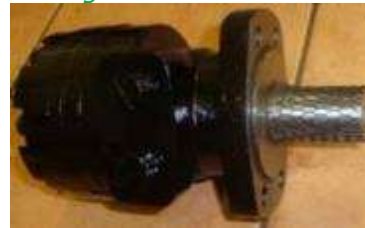
Hyd motor TPF 375cc BMER-2-375-MS-RW 6blt flange 1" shaft 7/8UNF ports (from 2019) - MHC BMER23754B1S $811.75 + GST
