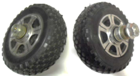
Rear Air free wheel, aluminium rim 220 OD with 20 x 140mm bolt axle with 6204.2RS heavy bearings & grease nipple (from 2019) – ZWBSWA210x60
