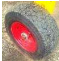
Front wheel 16-650-8" 30mm centre air free – ZVS8 Front wheel seal protector 30mm centre wheel – BWZFM27X60X30X4
