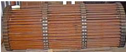
Belt: riveted bar conveyor 4 belt, 40 pitch, hi-profile, 250 12mm bars 1500 wide – WBRBC4BELRD
