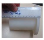
four large self lubricating HDPE bushes each 120mm long x 8mm thick with 10mm flanges.
