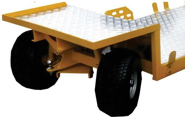
connects the front steering to the back wheels, which steers the rear wheels slightly sharper. This system stops the trailer cutting in on corners. The draw-bar is fitted with a 50mm ball hitch, the rear of the trailer is fitted with a 50mm ball. Multiple trailers can be towed behind each other following in the same path.
