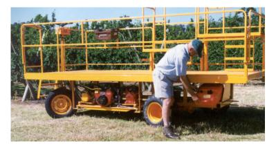
Trel-Pick is powered by a 14hp V-twin petrol engine with oil alert and has a large air compressor able to run four air secateurs. The engine base is mounted on springs to reduce vibration. A 25 litre remote fuel tank can be removed for easy refuelling.
