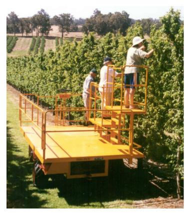
A towing hitch enables a bin trailer to be towed behind the Trel-Pick for use by ground pickers.
