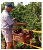
Four crate holders are standard which hold a 22 It or 36 It crate. This holder fits over the hand rail.
