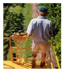
The Trel-Pick is simple to drive. The operator has control over engine throttle, hydrostatic ground speed, power steering and engine start and stop.
