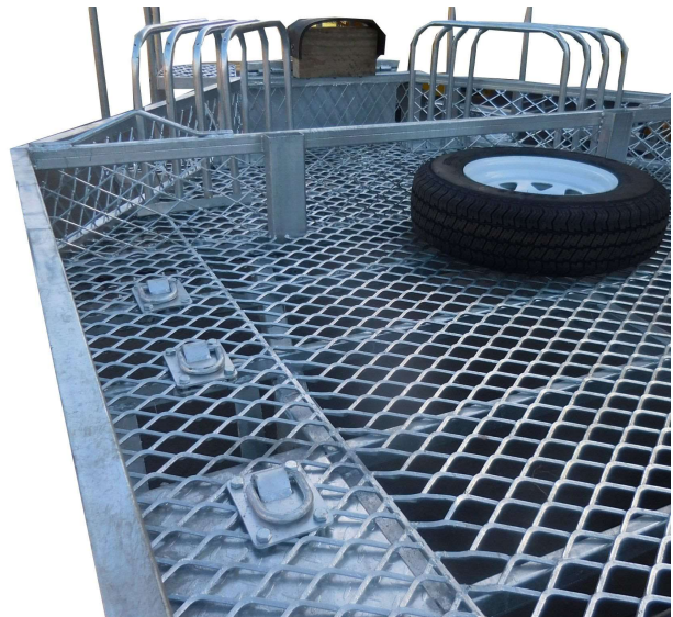
Floor is 6mm floor mesh with Heavy tie down lugs in floor
