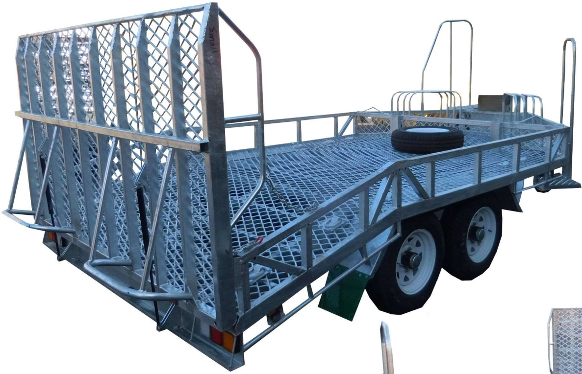
Rear ramps assisted by 2 Gas struts Side frame on ramp and trailer provide strength and safety
