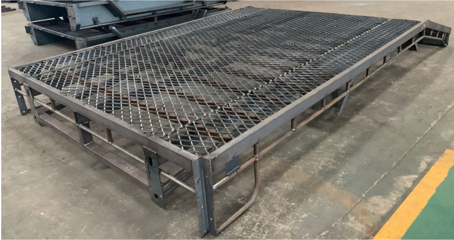
Tray ready for welding
