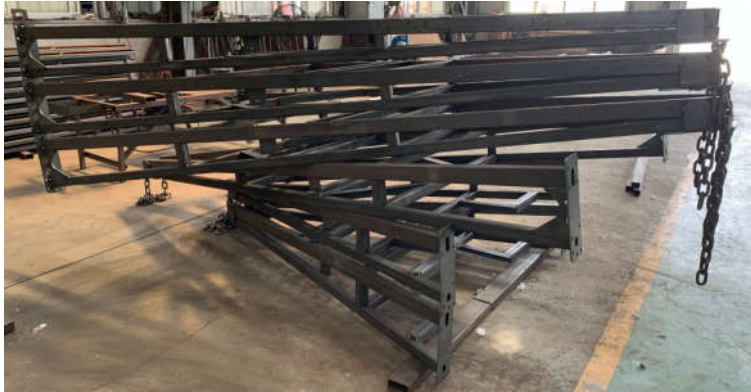
Drawbars ready for welding, Medium on top Short on bottom
