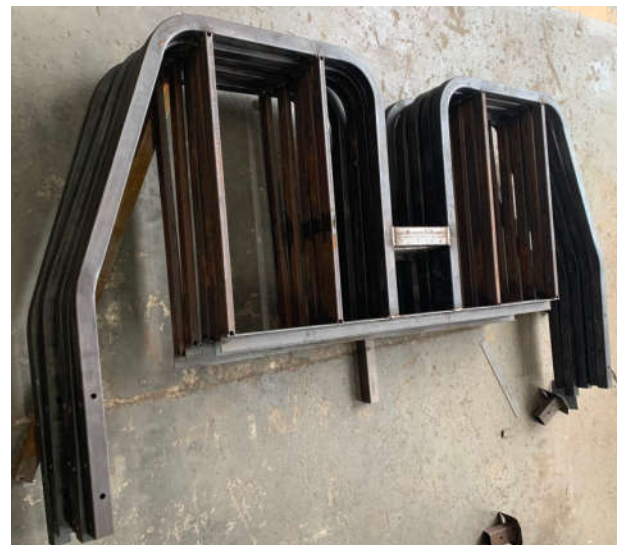
Head frame ready for welding,
