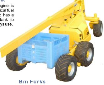
Bin Forks with a maximum load of 600kg are standard on all 4 models and is operated from the cage.
