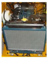
Kubota diesel engine 23hp 3 cyl water cooled
