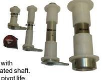
Caster wheel and bogie rocker pivots are Ø75mm shaft. Boom pivots are Ø50mm shaft. Boom lift ram pins are Ø40mm shaft. Stabiliser Bar & Cage Side Swing pivots are Ø30mm shaft.
