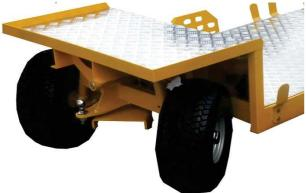
connects the front steering to the back wheels, which steers the rear wheels slightly sharper. This system stops the trailer cutting in on corners. The draw-bar is fitted with a 50mm
