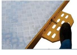
with your foot when required. As soon as the trailer is moved these swing back up. These steps are positioned in the centre of each bin are not in the way when unloading with a fork-lift. Side steps can be unbolted and removed if not required.
